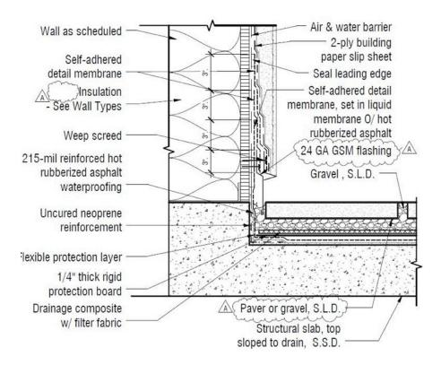
While the overview of this detail may appear more confusing than that of the incomplete detail above, the enlarged detail will show that this detail is complete and accurate.
