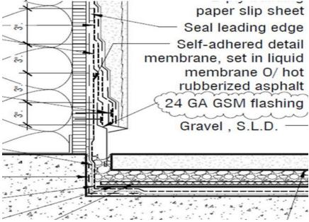
Notice how this detail shows clearly the various layers of flashing and how they are integrated (lapped). In addition, all other graphic elements, including arrows, are clearly visible.
