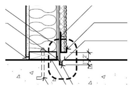
In this close-up example, the integration of the components shown becomes confusing as graphically the weather-resistive barrier, indicated with dashed lines, and the continuous galvanized metal flashing, a thin vertical line, merge with the thick black line of the J weep screed. In addition, the arrows get lost. Now see the difference in the next example of complete details:
